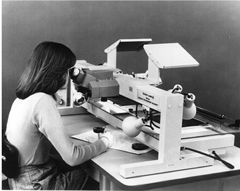
Figure 1. An example of the Bausch and Lomb Zoom transfer Scope used for capturing the boundaries of the estuarine habitats for the West et al. (1885) report. (Image source – The Remote Sensing Tutorial, http://geoinfo.amu.edu.pl/wpk/rst/rst/Sect15/Sect15_3.html )
